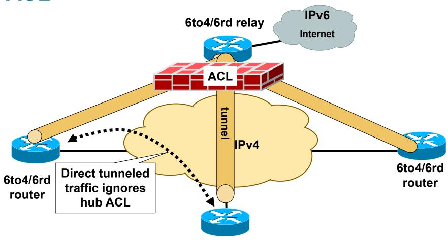
6rd CPE router can be configured to always go through hub Direct CPE-CPE communication must then be forbidden by IPv4 network
